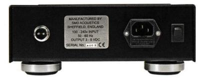
A two pin screw connector delivers power to a 1.4 metre fabric covered power cable. Mains power input was via a conventional IEC connector, the Maxon control board accepting 100V-240V mains input.
